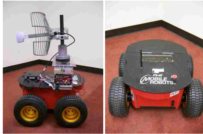
Figure 2.2: (left) Pioneer 3-AT robot equipped with a servo mechanism and a directional antenna. (right) Pioneer 3-AT robot equipped with an omnidirectional antenna.
