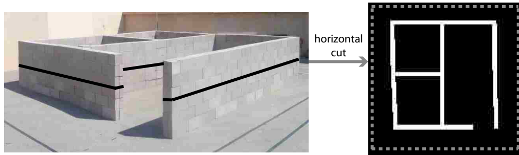
Figure 5.15: (left) The obstacle structure of interest and (right) its horizontal cut. The paths where the robots can make random wireless measurements are marked with dashed lines in the right figure.
