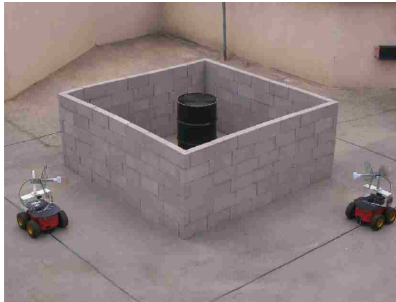
Figure 4.6: (left) Two pioneer 3-AT robots equipped with our servo control mechanism/fixture and an adaptive narrow-beam directional antenna in action, making wireless measurements in order to map the obstacle.
